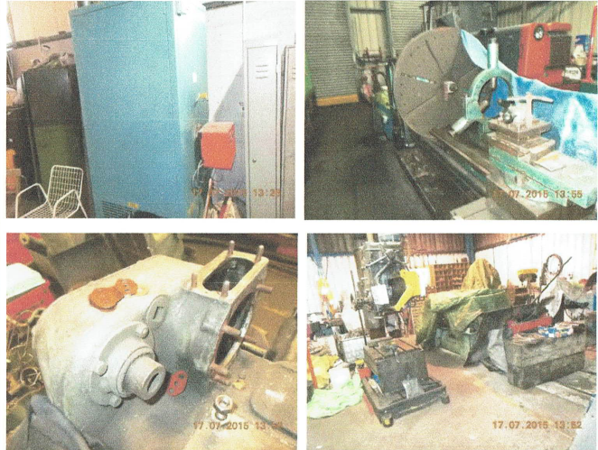
Older machinery may contain asbestos in the form of gaskets
